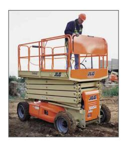
Full-time automatic traction control and an oscillating axle boost off-slab productivity.
